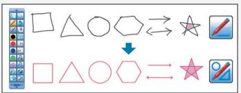
You can automatically convert freehand shapes into geometric objects and handwriting into text on the projected image using the StarBoard Software. These operations are easily accomplished with the interactive pen.
